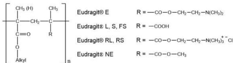
Fig. 2. Chemical structure of polymers used in the development of ocular drug delivery systems.
